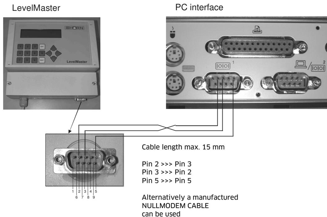
ill. 7 Wiring diagram for LevelMaster with zero modem cable
