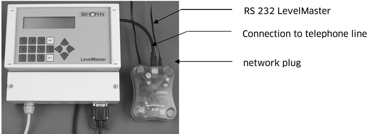
ill. 9 Wiring diagram for LevelMaster with landline modem
