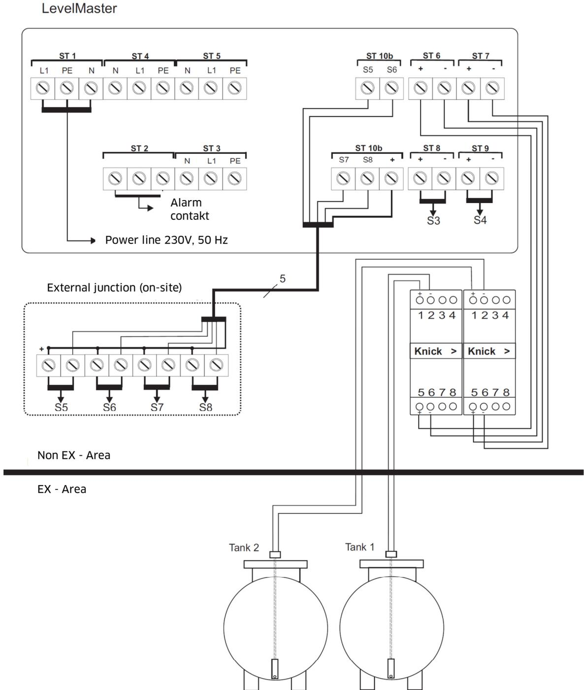
ill. 5 Connection plan for LevelMaster with passive repeater transmitter (example for two tanks)
