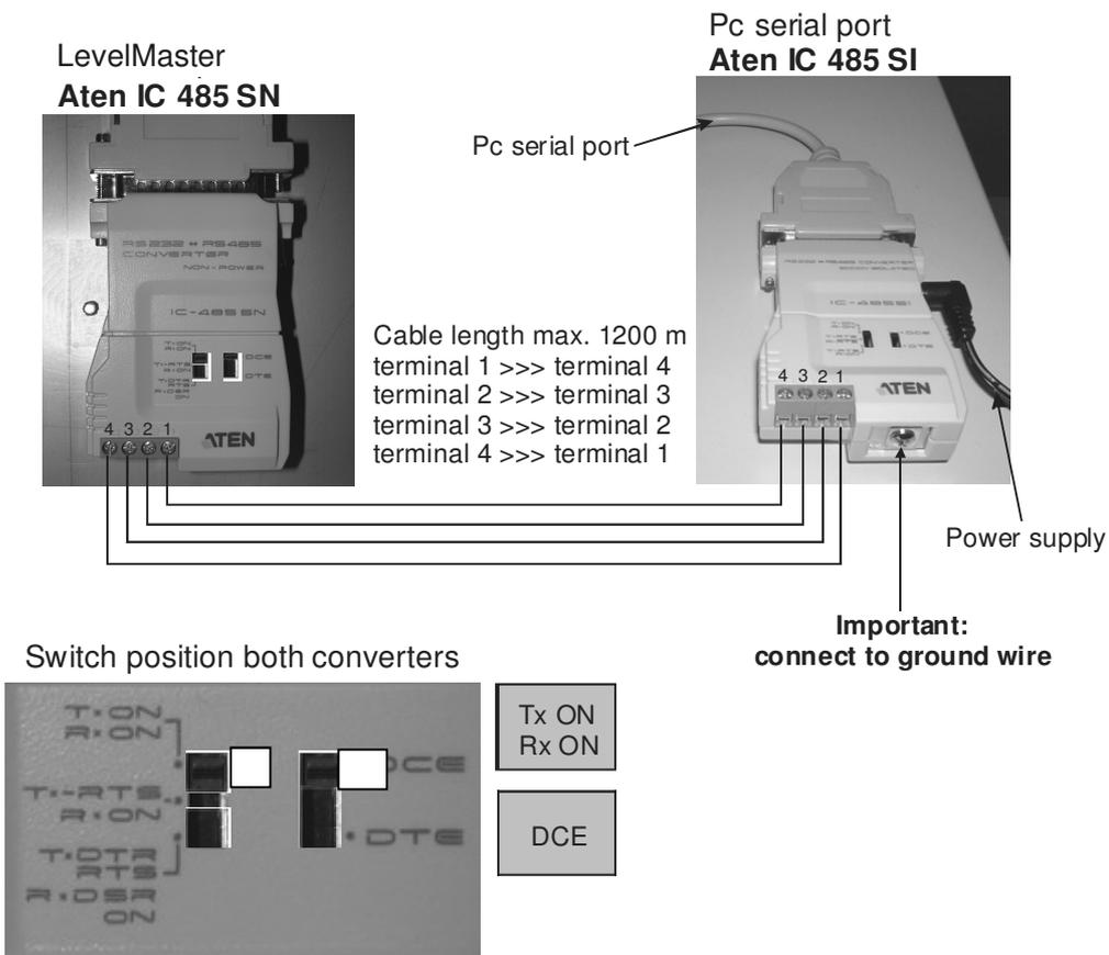
ill. 8 Wiring diagram for LevelMaster with converter set
