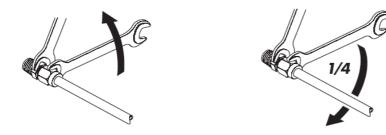
5. Checking of fit: Release the union nut completely. A distinct bead or deformation must be visible on the inside of the tube. It is of no detriment to the efficiency of the connection if, after assembly, the ferrule can be turned on the tube, or the tube in the union nut.
