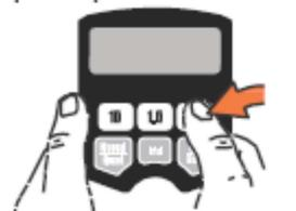
**Press the Manual / Reset key to reset the display to 0.00.**
