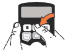
And press the 0.1 key to modify the first digit after the decimal point. The value zero cannot be input.
