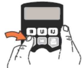
2. Press and hold down the Manual / Reset and Auto / Reset keys simultaneously for approx. six seconds to enter the configuration menus.
