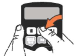
And press the 0.1 key to modify the first digit after the decimal point. The value zero cannot be input.
