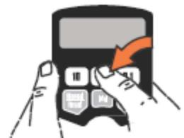
And press the 0.1 key to modify the first digit after the decimal point. The value zero cannot be input.
