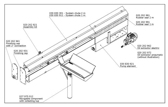
To avoid the pollution of the chute system, a special, retrofit able rubber seal can be fitted into it.
