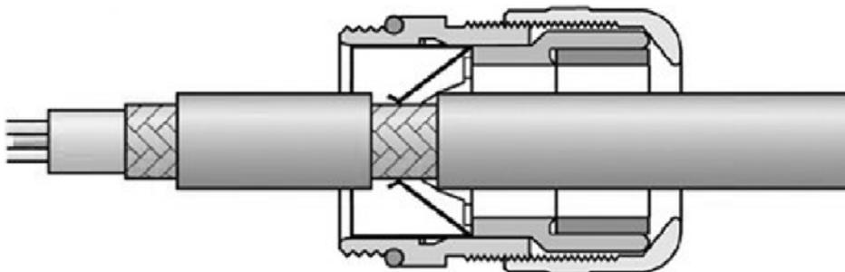
**!** **Shielded cables must be used for the control cable of the flow meter and the data cable. Otherwise a negative effect of the function can occur and damages or malfunction can happen.**
